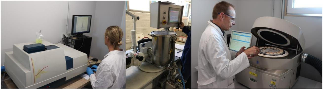
**Figure:** German Piloting Equipment (L - R) Laser Particle Sizer, Micronising Mill and Thermo Gravimetric Analyser
