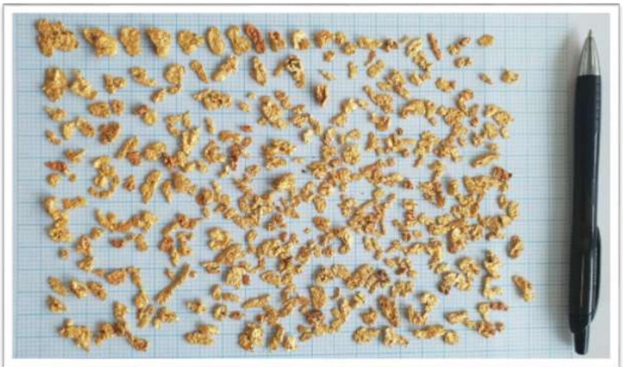
Figure 1. Coarse gold nuggets recovered from an alluvial “trap-site” downslope of Bellary Formation conglomerates.
