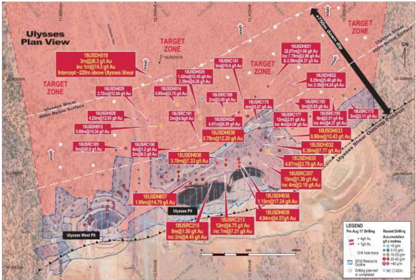
Figure 1. Plan view in local grid showing new intersections from recent diamond and RC drilling in yellow text and previously reported 2018 results in white text. The Ulysses shear dips at ~35 to 30 degrees to the north and for this reason it is visualised best in plan view. Approximate positions at surface – outcrop, 200m below surface and 400m below surface of the Ulysses Main shear are shown. The circles and diamond shapes are pierce point positions (intersection points) on the Ulysses shear or on splays off the main shear. The dark blue outline is the boundary of the 2018 Mineral Resource in plan view. True widths are ~90% to 100% of down-hole lengths.
