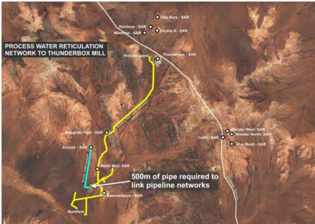
Figure 2 – Process water reticulation from Sinclair to Thunderbox mill (500m LINK ONLY REQUIRED)
