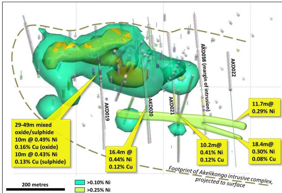
Figure 2. Drill plan at Akelikongo, (purple dotted outline marks outline of intrusion) showing results from AKD018-22 reported ASX 20 June 2019 and new eastern mineralised zone (schematic) shown in yellow.
