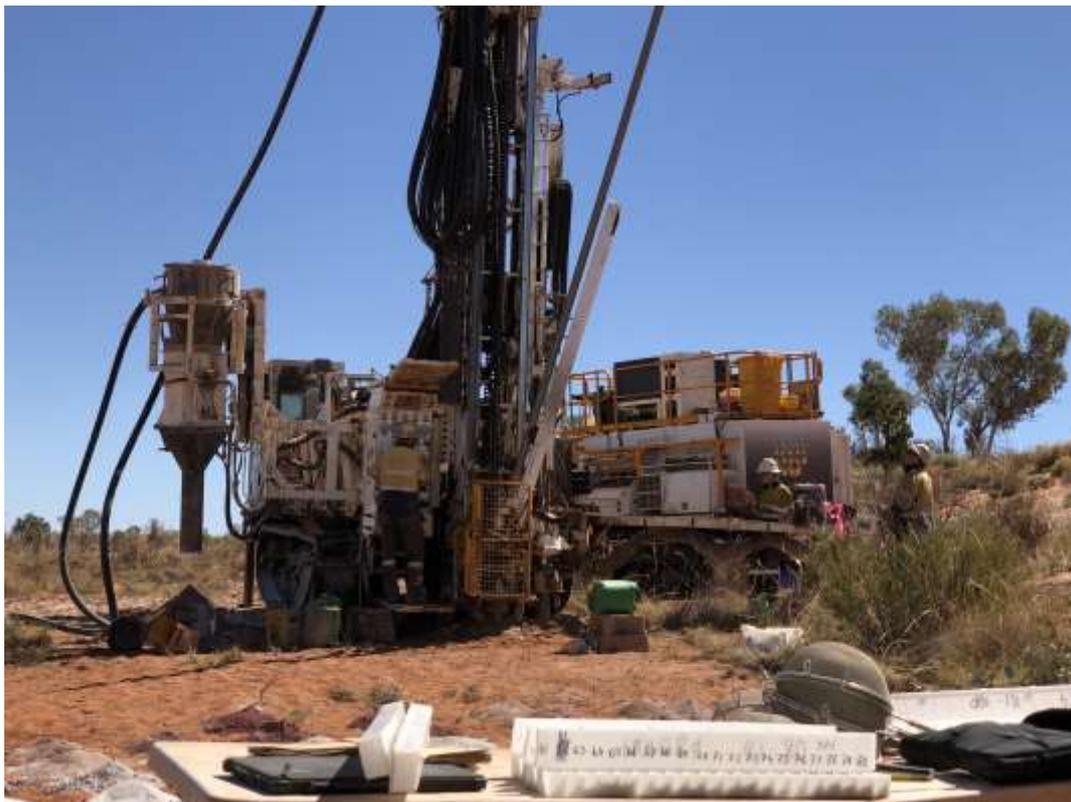
*Strike Drilling track-mounted Aircore /RC rig drilling at Obelisk, Paterson North, Western Australia*
