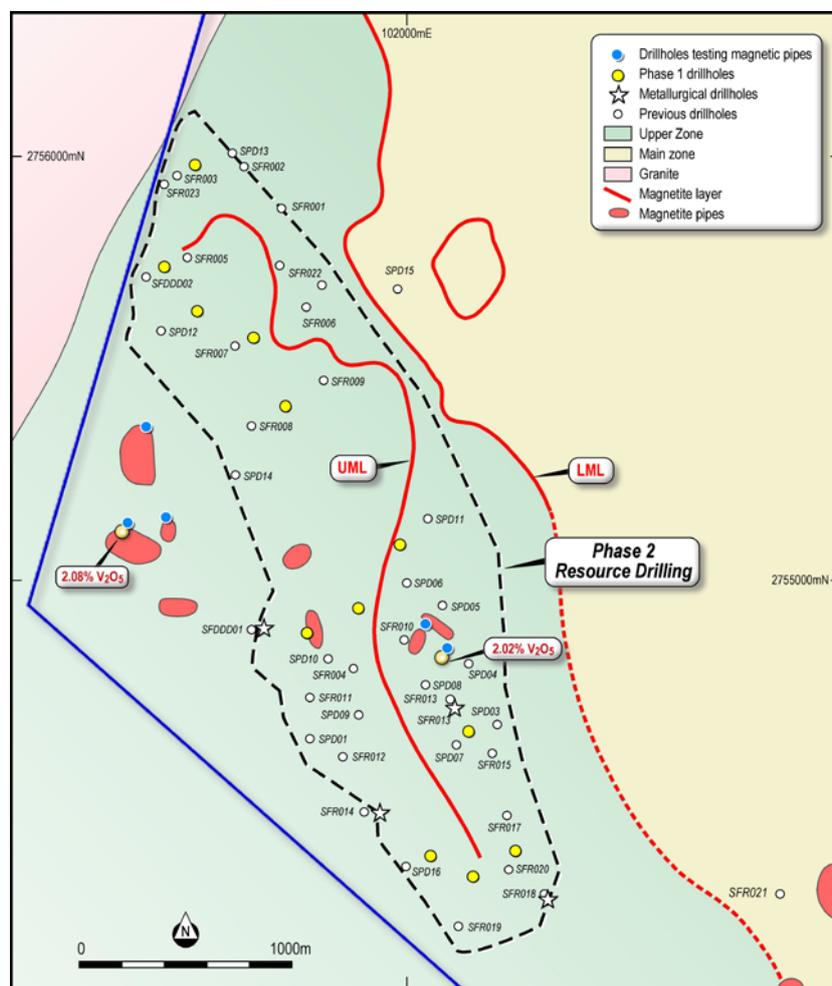
**Figure 1.** Phase 1 and Phase 2 drilling planned for the SPD Vanadium Project.
